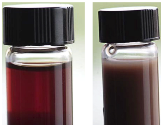
Figure 2. Picture of the clarified vinasse (on the left) and of the effluent (on the right).
